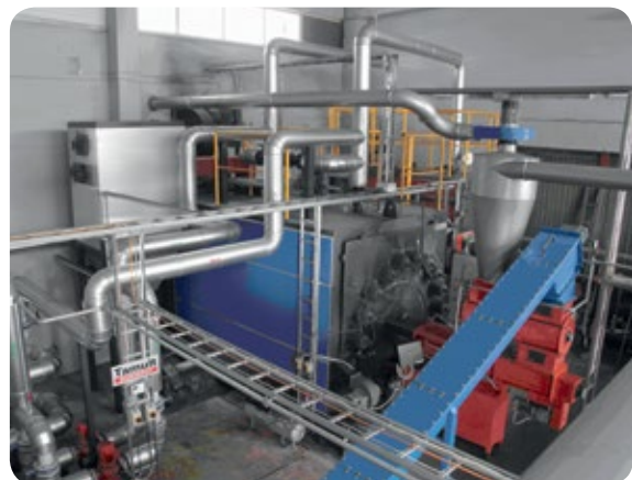
Figure 6: Transporter (left) and combustion chamber (right) of the facility for burning crushed (scarified) straw and reed. (Photos by Ü. Kask)
