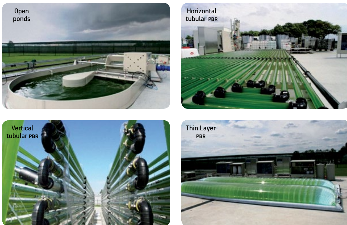
Figure 6: Four different types of photobioreactors (pictures: AlgaePARK).
