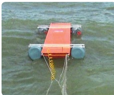
Figure 10: Floating device with installed linear movement generator.
